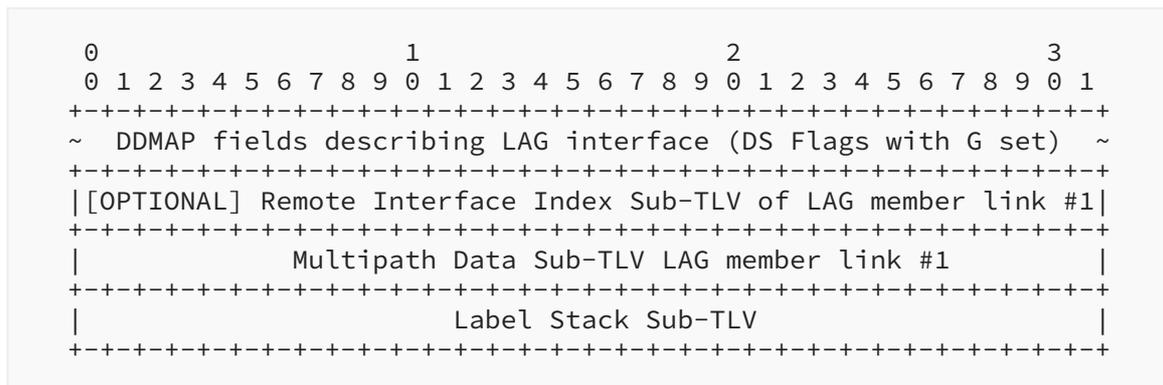
Figure 3: Example of DDMAP in MPLS Echo Request
