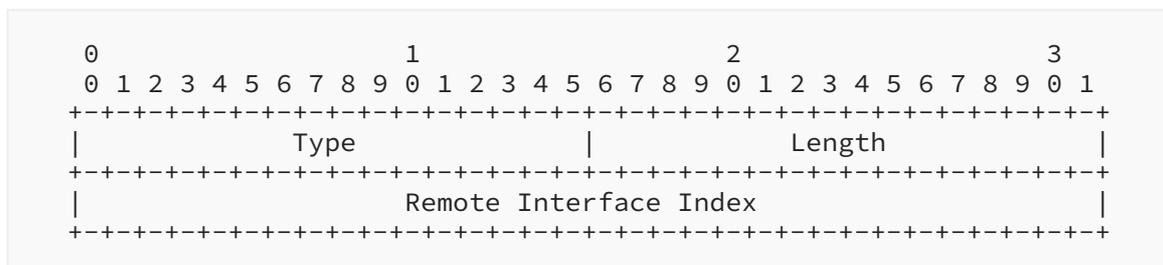
Figure 6: Remote Interface Index Sub-TLV
