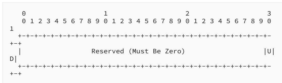
This document defines two flags. The unallocated flags MUST be set to zero when sending and ignored on receipt. Both the U and the D flag MUST be cleared in the MPLS echo request message when sending and ignored on receipt. Zero, one, or both of the flags (U and D) MAY be set in the MPLS echo reply message.
