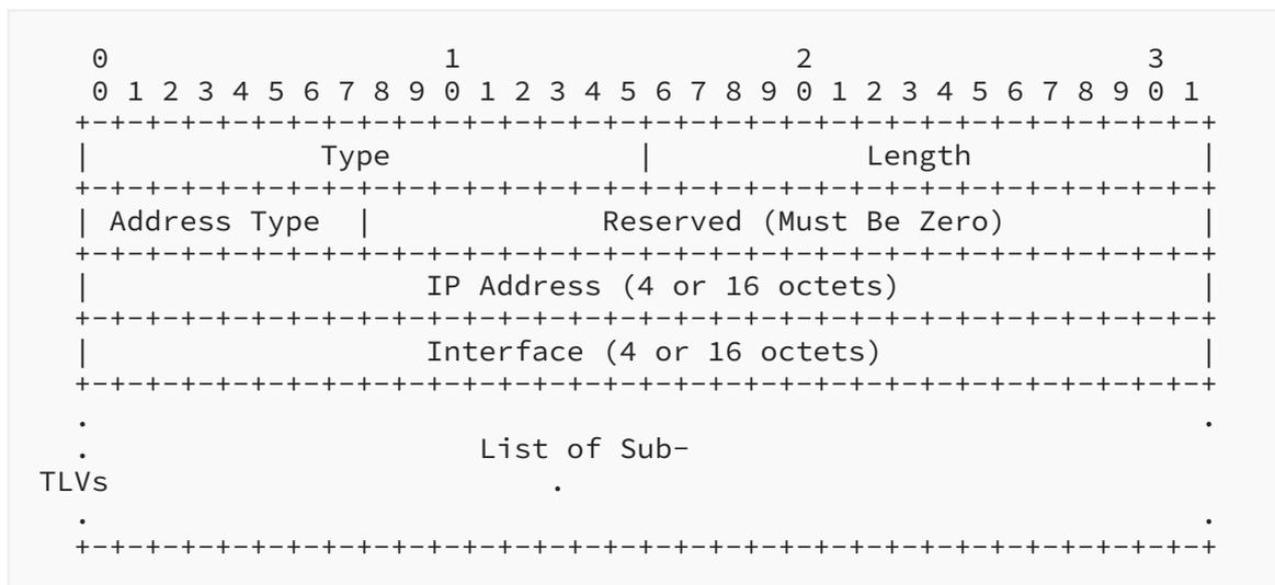
Figure 7: Detailed Interface and Label Stack TLV
