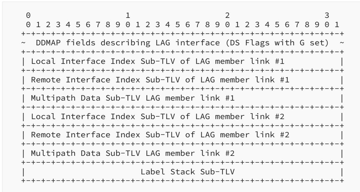
Figure 2: Example of DDMAP in MPLS Echo Reply
