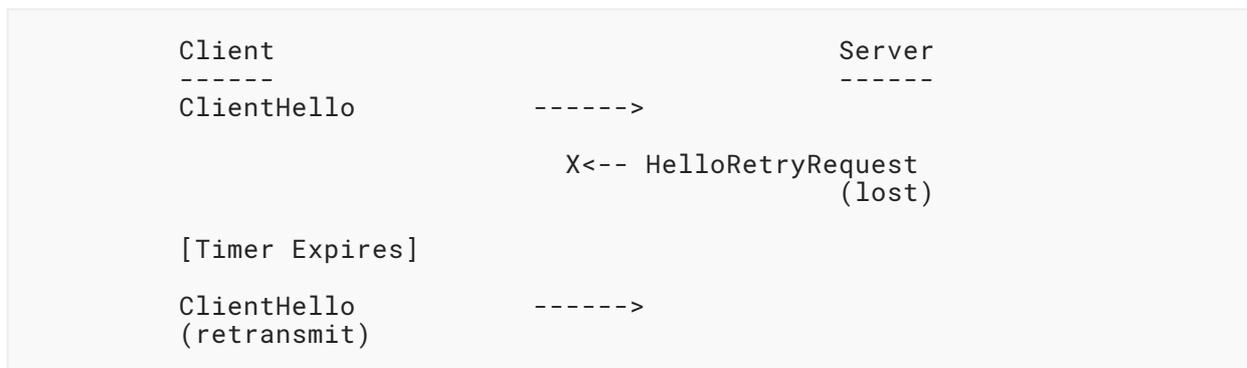
*Figure 1: DTLS Retransmission Example*
