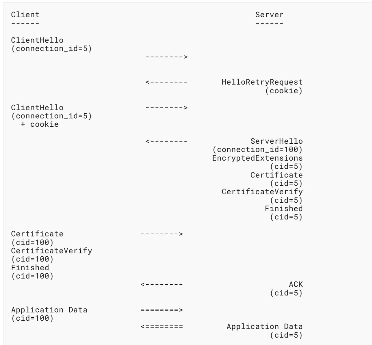
Figure 15: Example DTLS 1.3 Exchange with CIDs
