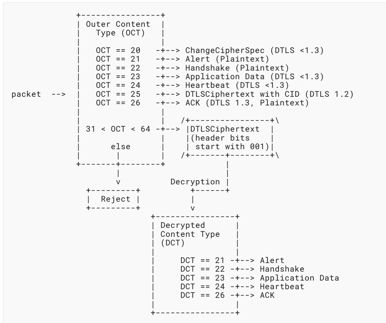
Figure 5: Demultiplexing DTLS 1.2 and DTLS 1.3 Records
