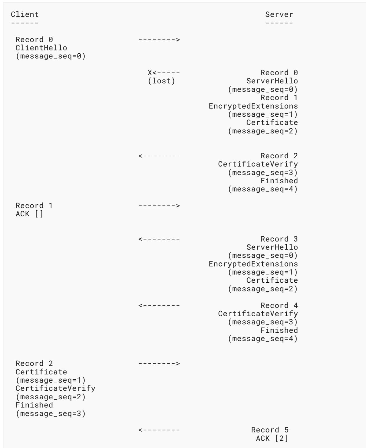
Figure 12: Example DTLS Exchange Illustrating Message Loss
