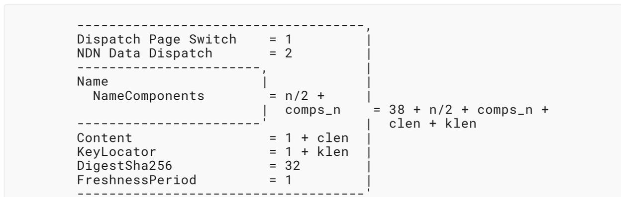
Figure 37: Estimated Size of a Compressed NDN Data
