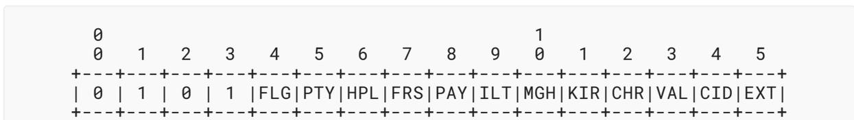
Figure 21: Dispatch Format for Compressed CCNx Interest Messages
