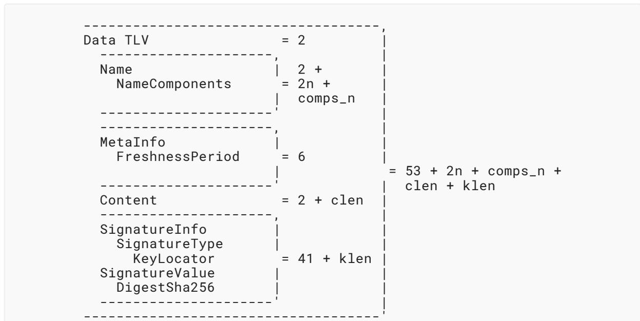
Figure 36: Estimated Size of an Uncompressed NDN Data
