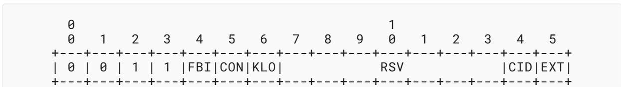
Figure 17: Dispatch Format for Compressed NDN Data Messages
