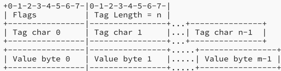
Where  $n$  is the length specified in the Tag length field and  $m$  is the remaining octets in the Value field. They are related by  $(m = d - n - 2)$  where  $d$  is the length of the RDATA section.
